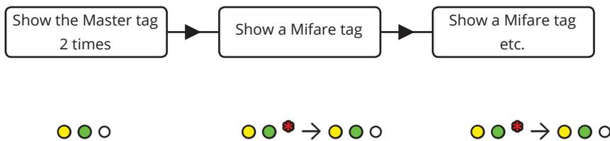
The M1000 can also delete all users at once, delete a lost user and delete the master transponder. Use the enclosed configuration scheme as a guide.
