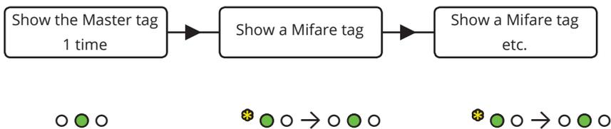
To exit the programming, wait for 30 seconds or disconnect and reconnect the voltage.
